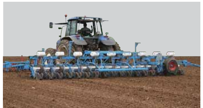
18-row rigid triple bar MECA V4 planter with Microsem and transport carriage
