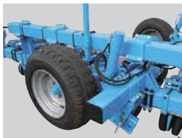
A lengthwise transport carriage (for TIP 5" frame) is available for wide configuration planters. This transport carriage may be with manual or hydraulic lift.
